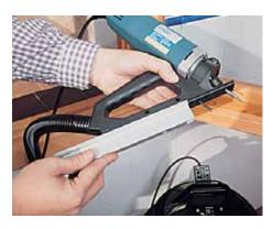
Equipped with 2 types of interchangeable fences which allows you to make slots at 45° angle or straight.
