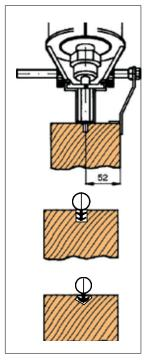
Using the straight fence and reversible square, slots on smooth areas such as the side of door hinges.
