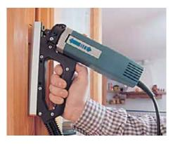
With centering pivot easing entry of the bit at the start of the slotting process.
