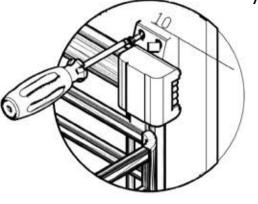
1. Fix to mechnanism leaving a distance of 10mm from the front of the carcase to the start of the connection plastic mechanism as shown in diagram (A-1).
