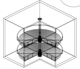
Step 5: Adjust the height of basket and fix it with the boles , then screw the plastic parts.
