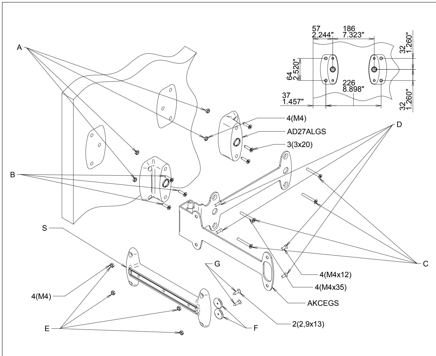
1. Insert the nuts "A" in the base of the support AD27ALGS.
